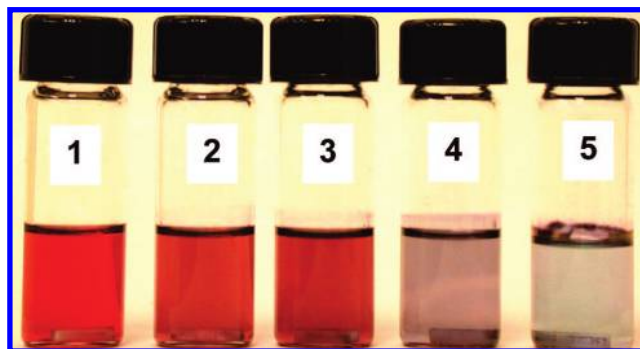
Figure 3. Photograph of Au NP dispersions, which aggregated when the concentration of Pc 4 was increased in chloroform. Vial 1 was pure Au NPs as control. From vial 2 to vial 5, the [Pc]/[Au NP] concentration ratios were 20:1, 40:1, 50:1, and 60:1, respectively.
